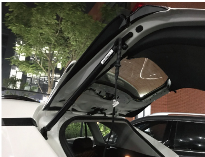
Route strut cable in factory holes in door panel
