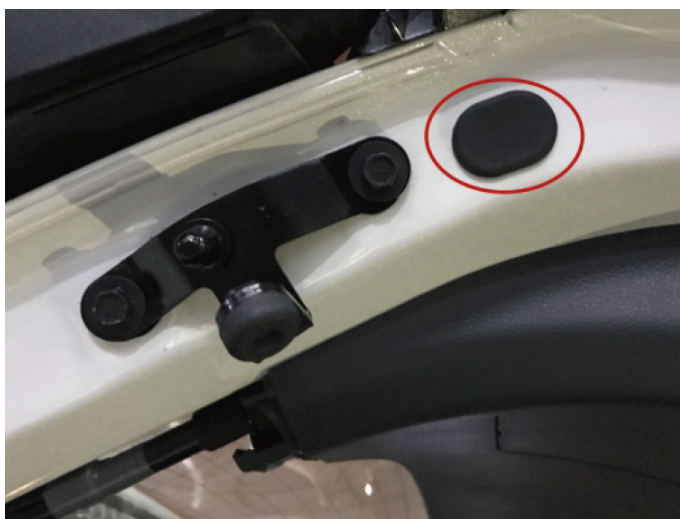
Route strut cable in factory holes in door panel
