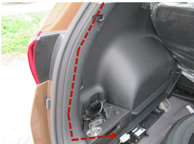
Route power cable to driver's position, route green wire to B pillar, picture for reference only
